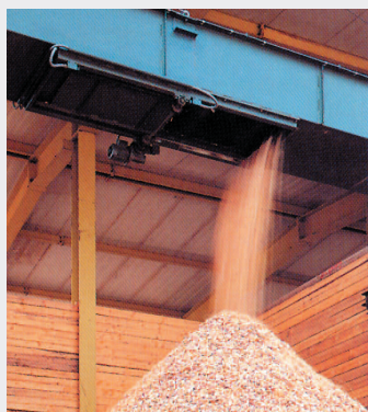
Drag Chain Conveyor KKF 970-2K-0 for loading and leveling trailers and containers
