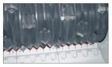
Counterknife standard tolerances are .015 to .020 clearances. Options are available for clearances to .010.
